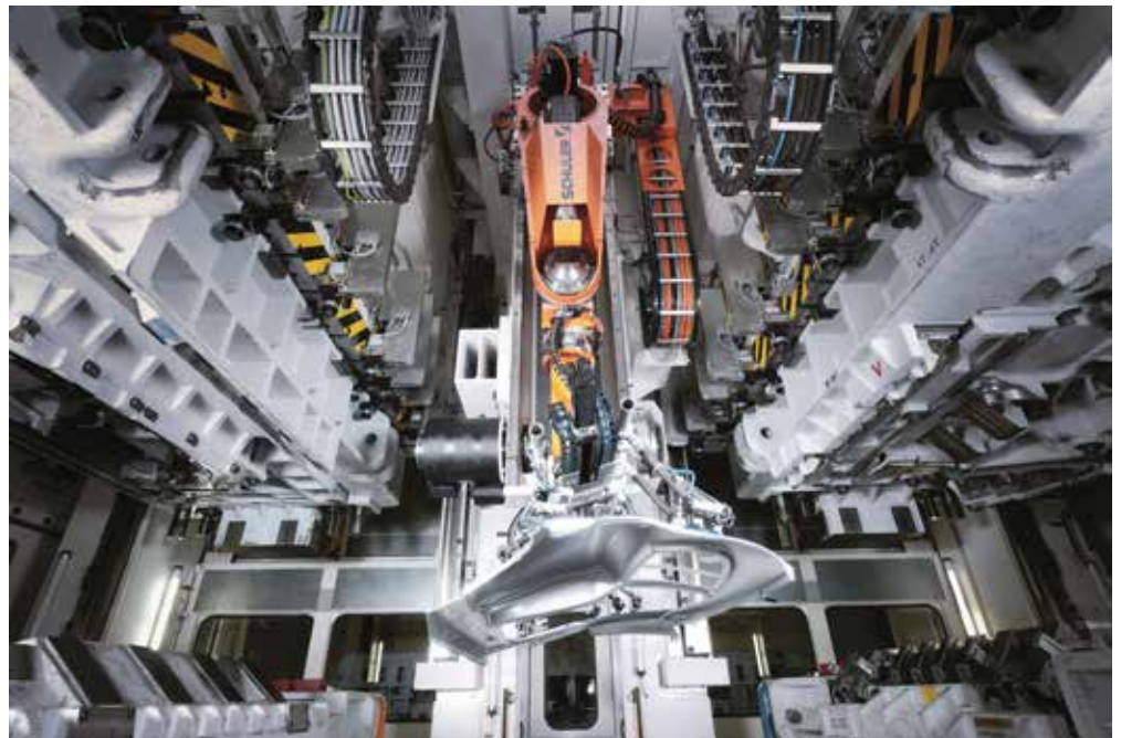
Automated robot from Company Schuler transport for instance for a car body
